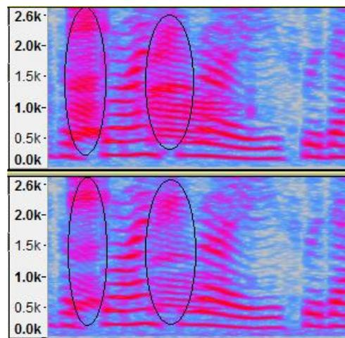
Figure 2 : Double-talk segment before DMA (top) and after DMA (bottom).
