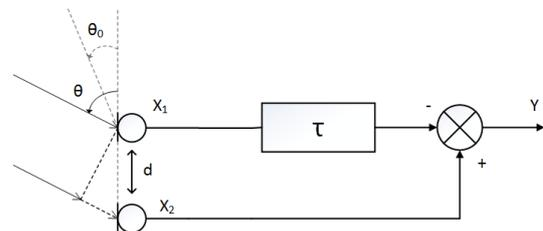
**Figure 1 : Block diagram of a differential microphone array with 2 microphones**
