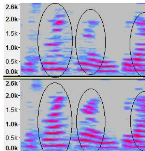
Figure 3 : Double-talk segment processed by the echo postfilter standalone (top) and double-talk segment processed by DMA and echo-postfilter (bottom). The circles show the near-end speech component.
